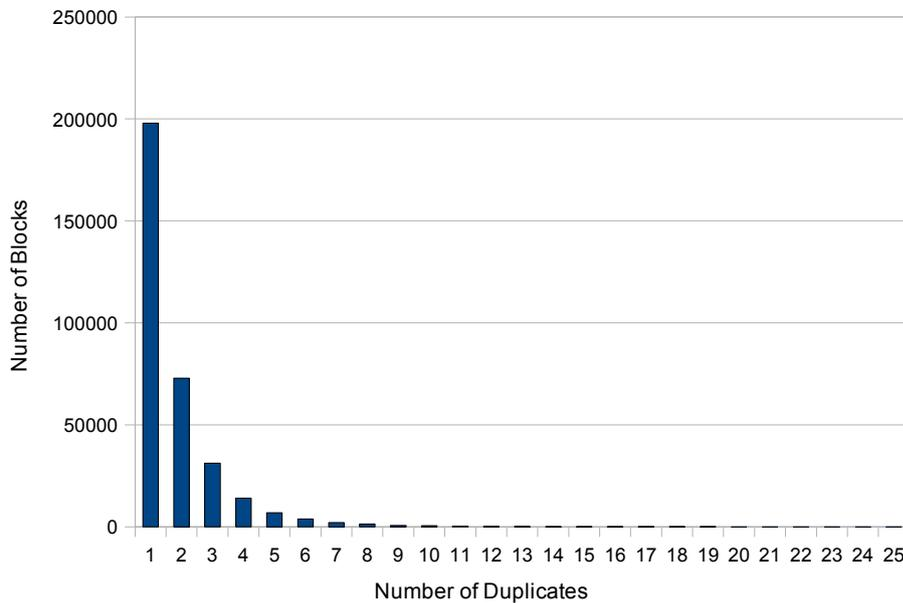
Figure 6.2: Redundancy distribution: Blocks with less than twenty five duplicates.
