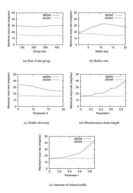
Figure 3: Impact of group size, buffer size and traffic profile in maximum throughput.
